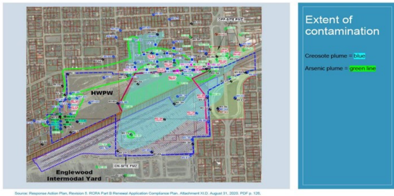
Figure 2 Map of extent of contamination that shows the old Houston Wood Preserving Works (HWPW) facility within the dashed blue outline. Creosote plumes (light blue shading) extend beneath the neighboring houses to the North of the facility, and the arsenic plume (green line) also extends beneath the neighboring houses close to the facility.
