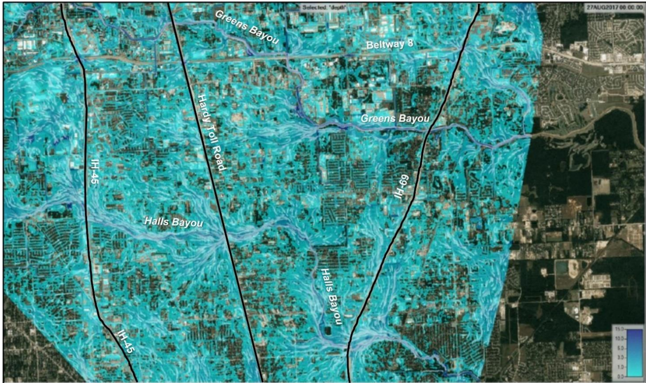
Figure 10. HEC-RAS modeling of flooding in the Northeast during Hurricane Harvey when over 25,000 homes flooded in the Greens Bayou Watershed. In this image, Greens Bayou is flowing across the upper part of the diagram, crossing the Hardy Toll Road before going under Beltway 8 and then flowing east under the Eastex Freeway. Halls Bayou is shown crossing the middle portion of the image under IH 45, the Hardy Toll Road and the Eastex Freeway. Image courtesy of Dr. Phil Bedient, SSPEED Center, Rice University.
